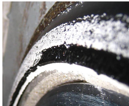
Fig. 14. Photograph showing the wear zone of the lip-seal
