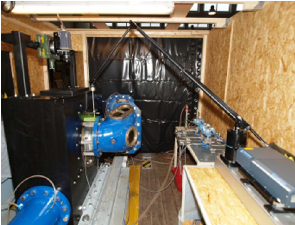
Test rig with Laser installation
